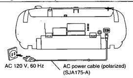
If the unit is not going to be used for a prolonged period of time when a household AC outlet is used to power it, disconnect the power cable to conserve power.
